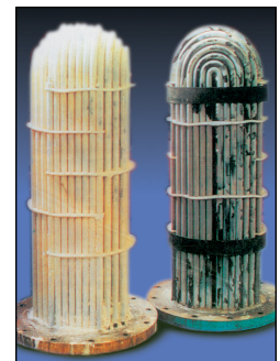
Encrusted Heat Exchangers
