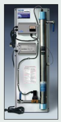
TWT-UVC-3000 (30 GPM) Ultraviolet Disinfection/Purification System Mounted on St/St frame with Manual Shut-Off Valves, Alarm, UV Monitor and Automatic Solenoid Valve • Size: 20"W X 55"H 10"D Available 120V/60 Hz or 230V/50 Hz
