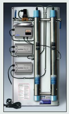
TWT-UVC-5000 (50 GPM) Ultraviolet Disinfection/Purification System Mounted on St/St frame with Manual Shut-Off Valves, Alarm, UV Monitor and Automatic Solenoid Valve • Size: 25"W X 55"H 10"D Available 120V/60 Hz or 230V/50 Hz
