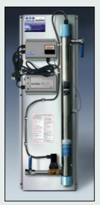
TWT-UVC-1500 (15 GPM) Ultraviolet Disinfection/Purification System Mounted on St/St frame with Manual Shut-Off Valves, Alarm, UV Monitor and Automatic Solenoid Valve • Size: 20"W X 55"H 10"D Available 120V/60 Hz or 230V/50 Hz
