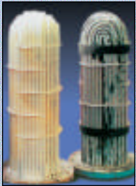
Encrusted Heat Exchangers
