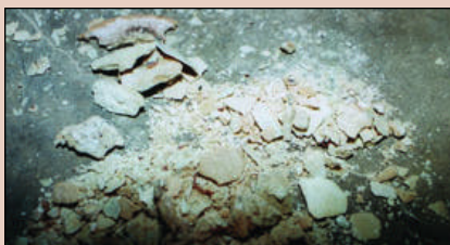
Pounds of Scale Removed from a Hot Water Plumbing and Heating Systems
