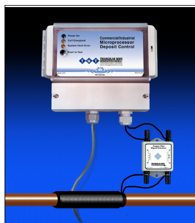
TWT-Deposit Control Solenoid Coil Wrap with a CSE Copper Pipe Signal Enhancer Application: Copper pipe signal enhancer is required for copper pipe applications only
