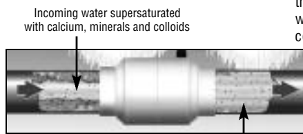
Conditioned water with minerals, colloids treated and the calcium converted to aragonite crystals
