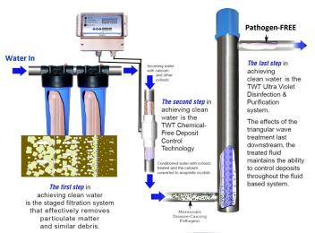
**Filtration**: Filters are designed to trap, remove and treat various kinds of debris and other organic particles and pollutants in the water. Upon request, filters are available in a variety of Media and Micronic sizes providing flexibility and adaptability to meet the needs of almost any water condition or application. Double (10" BB) filter housings, with sediment and carbon filters are standard.
