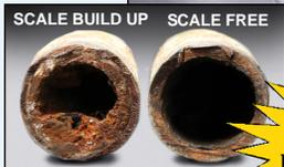
**ELIMINATE DEPOSITS IN PIPES, FIXTURES & EQUIPMENT**
