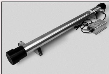
safe, potable drinking water, free of disease-causing pathogens. As water passes through the UV chamber, UV light will attack and render harmless any bacterial, viral or spore contamination present in the treated water. “High intensity UV light destroys these contaminants with a 99.9% or greater kill rate”. The output water is thus disinfected and offers exceptionally high quality for human consumption.
